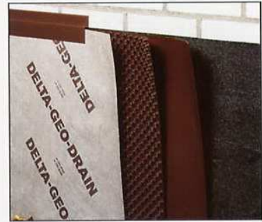
DELTA-GEO-DRAIN is a single erection element of three components bonded together in the factory: slip-layer membrane, dimpled sheeting, and geotextile durable filter.
