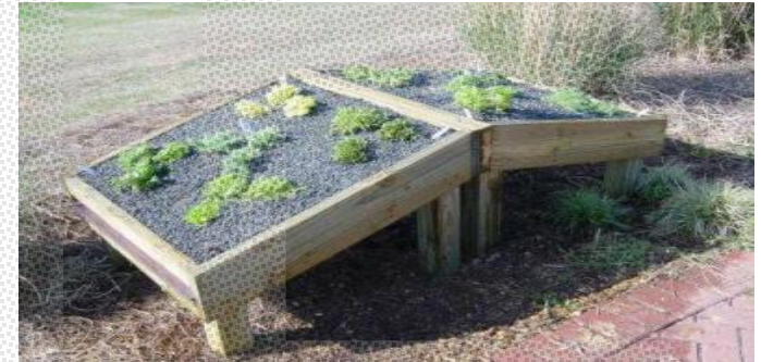
'extensive' green roof model, built at the Environmental Horticulture Department's ID Gardens, North Metro Technical College, Atlanta Georgia
