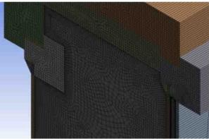
Fig. 170. – generic 3D box window with internal IG – swept inflation mesh for the frame adjacent portion of the cavity
