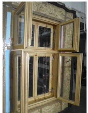
Fig. 21. – Window No. 3a – during temperature sensor installation
