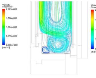
Fig. 227. – realistic 3D box window (window 2) – streamlines at the top of the cavity
