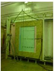
Fig. 7. – The surround panel at a separate stand with the calibration panel being installed
