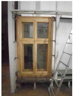
Fig. 20. – Window No. 3a – during airtightness testing in the window test rig
