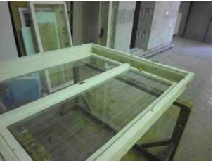
Fig. 14. – Window No. 2 – on a horizontal stand for temperature sensor installation
