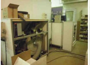
Fig. 3. – The pressurization (left) and temperature control (right) system of the window test rig
