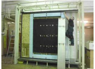
Fig. 6. – The cold side chamber being installed in the window test rig
