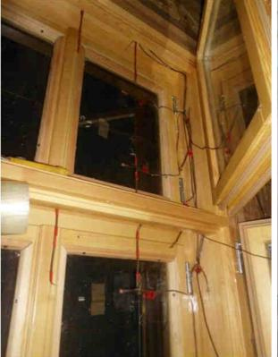
Fig. 22. – Window No. 3b – during temperature sensor installation
