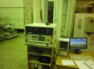
Fig. 4. – The control unit of the window test rig
