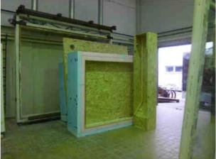
Fig. 1. – The components of the hot box before painting, assembly and instrumentation
