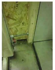
Fig. 9. – The seal between surround panel and the window test rig's wall with adjustable steel bolt
