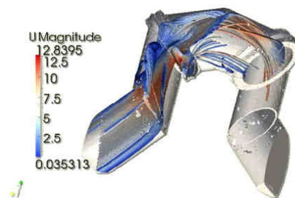
Images: Flow pattern inside the valve
